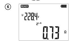
Read the main result: the fault loop impedance Z<sub>S</sub> and the mains voltage during the measurement.
