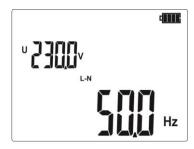
Read the measurement result: voltage in the auxiliary display field, frequency in the main field.
