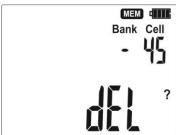
Set the bank number to • (before 0). The delt message appears, signaling that the meter is ready to delete.
